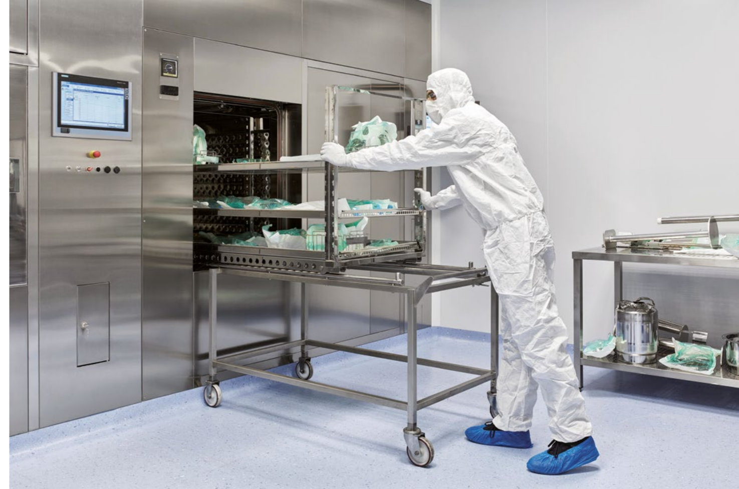
Aseptic operator loading tools for sterilization at CordenPharma Caponago (IT).
