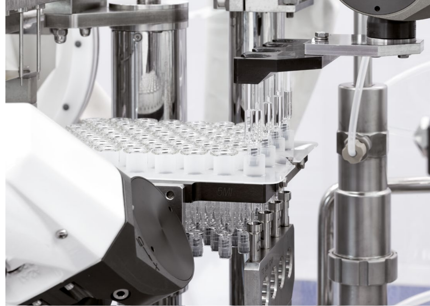
Pre-Filled Syringe robotized filling line and weighing / priming station at CordenPharma Caponago (IT).
