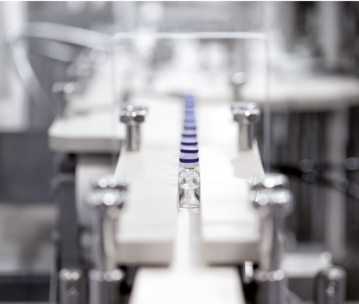
Aseptic filling line at CordenPharma Caponago (IT).
